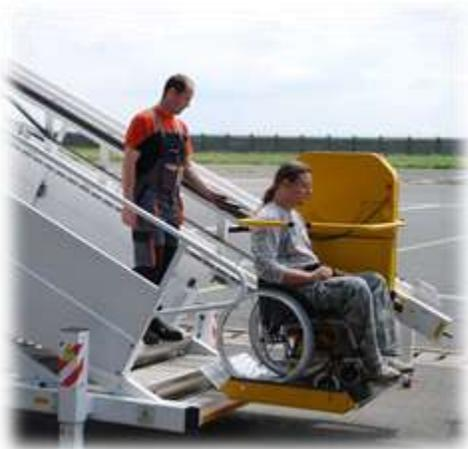
*Stairlifts allow passengers using mobility aids to board and exit an aircraft in a safe and comfortable manner.*
