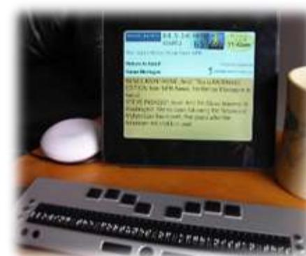
*A text-alert radio, with a refreshable Braille display*
